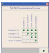
A PLC-PLC communication popup screen highlights any inter PLC communications failures.
